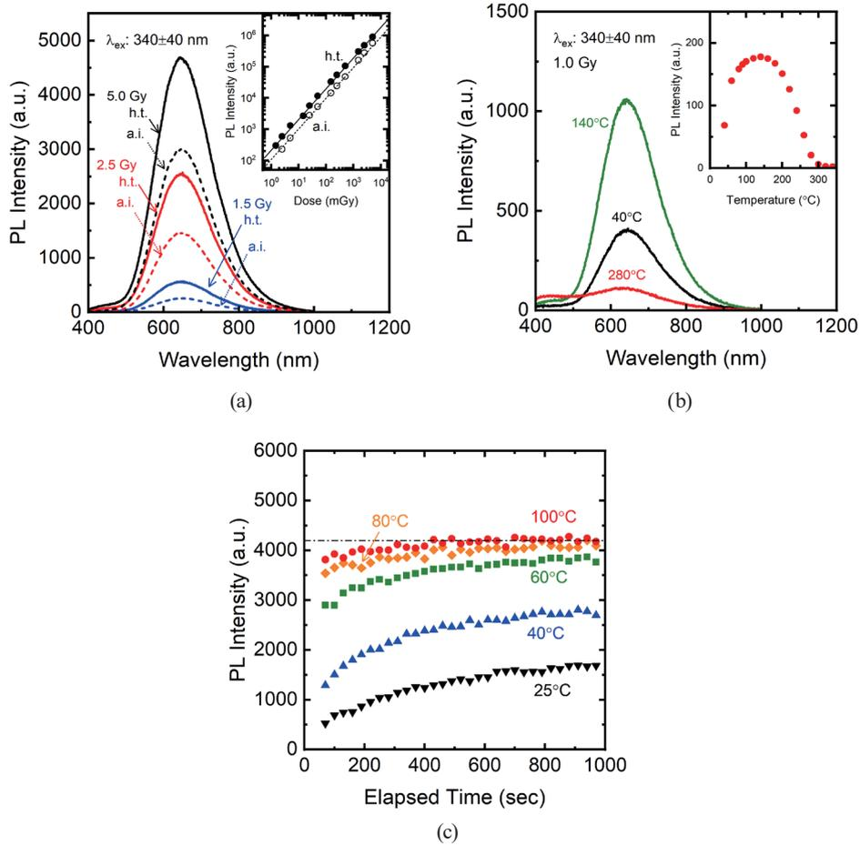
Fig. 6. (Color online) Example measurement results of RPL properties of Ag-doped phosphate glass (AGC Techno Glass). (a) PL (RPL) spectrum (as-irradiated, a.i.; heat-treated, h.t.) as a function of dose and dose response curves, (b) PL (RPL) spectrum and integrated intensity as a function of treatment temperature after irradiation and before measurement, and (c) PL intensity as a function of elapsed time after irradiation and storage temperature.
