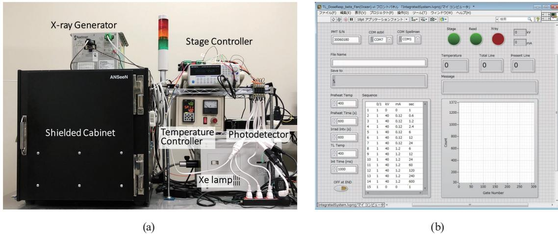
Fig. 2. (Color online) (a) Appearance of the prototype TORAIMS and (b) a controller program for TSL dose response measurement as an example.
