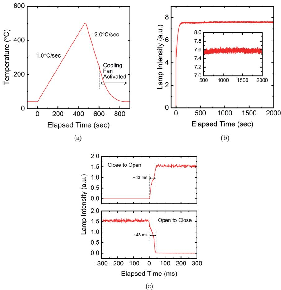
Fig. 3. (Color online) Demonstrations of (a) typical temperature profile during a cycle of TSL measurement, (b) stability of xenon lamp intensity, and (c) response of mechanical shutter.
