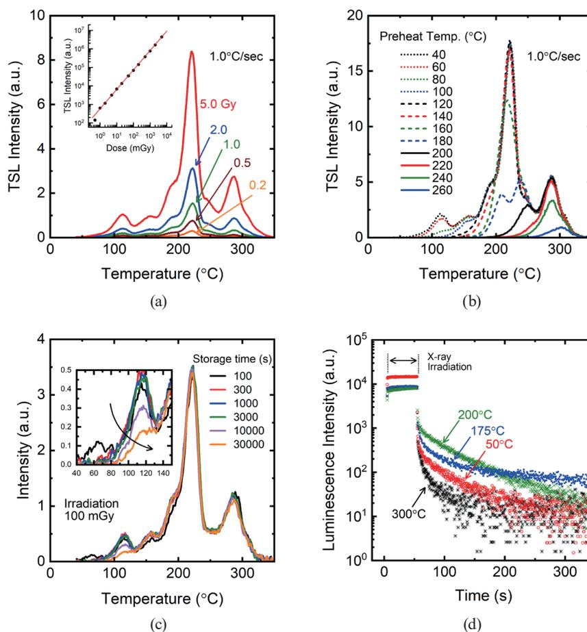
Fig. 4. (Color online) Example measurement results of TSL properties of LiF:Mg,Ti (TLD-100, Thermo Fisher). (a) TSL glow curve and dose response, (b) TSL glow curve as a function of preheat temperature, (c) TSL glow curve as a function of storage time, and (d) isothermal decay curve as a function of sample temperature.
