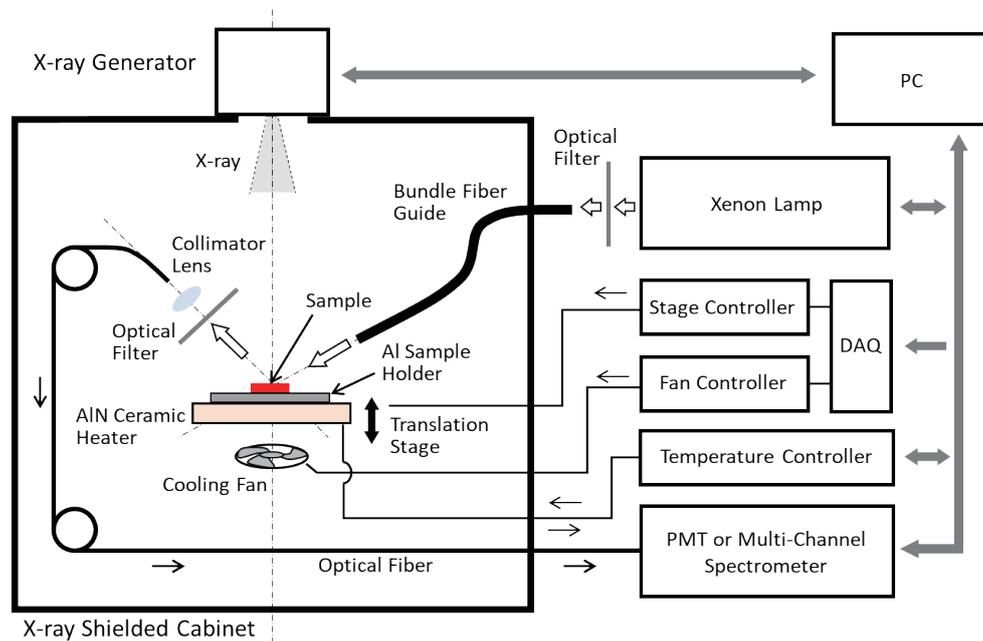
Fig. 1. (Color online) System configuration of the prototype TORAIMS (not to scale).
