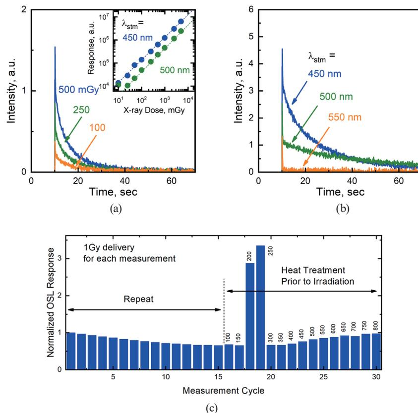
Fig. 5. (Color online) Example measurement results of OSL properties of BeO (Thermalox995, Materion). (a) OSL decay curves and dose response as a function of stimulation wavelength, (b) OSL decay curves as a function of stimulation wavelength, and (c) OSL response as a function of number of measurement cycles and treatment temperature prior to irradiation.
