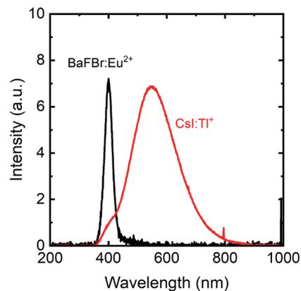
Fig. 7. (Color online) X-ray-induced scintillation spectra of CsI:TI<sup>+</sup> scintillator (Saint-Gobain) and BaFBr:Eu<sup>2+</sup> imaging plate (Fujifilm).
