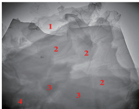
Fig. 6. (Color online) TEM image of GO, showing the existence of approximately four layers.
