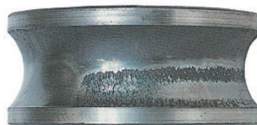
Fig. 6. (Color online) Inner raceway flaking.
