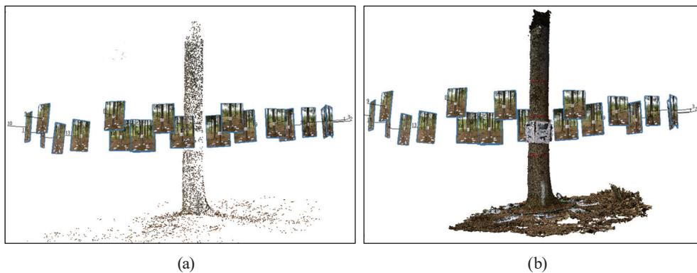
Fig. 6. (Color online) Reconstructed PCD of individual trees: (a) result of photo alignment and (b) visualization of reconstructed individual tree stem.
