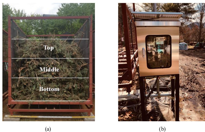
Fig. 1. (Color online) Metal frame with load cells (a) and data logging device (b) for weighing forest biomass during natural drying.
