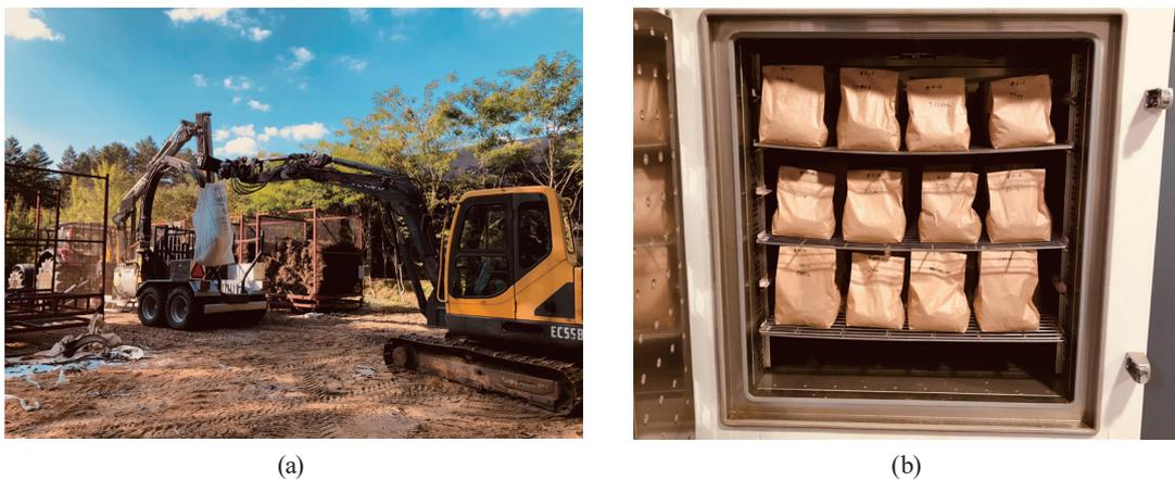
Fig. 3. (Color online) (a) Comminution of each forest residue pile and (b) oven drying of sample wood chip.
