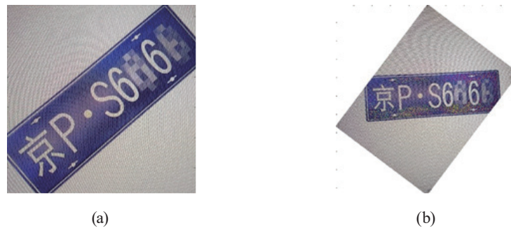
Fig. 9. (Color online) Correction of tilted image for license plate recognition. (a) Original image. (b) Corrected picture.
