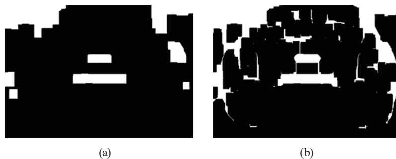
Fig. 3. (Color online) Edge detection result of license plate. (a) Original image of vehicle. (b) Image with closed operation.
