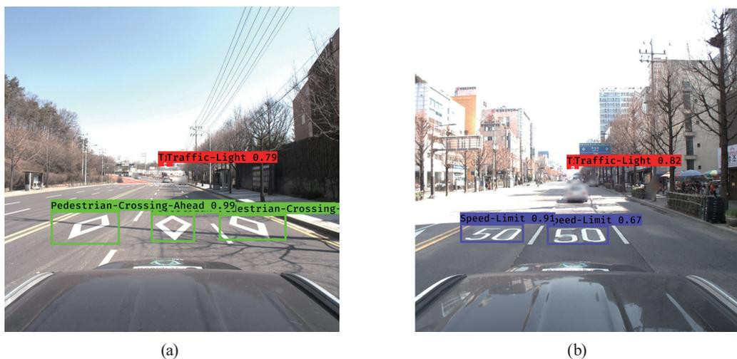
Fig. 6. (Color online) Road facility detection: (a) pedestrian crossing ahead and traffic lights and (b) speed limit road marks and traffic light.
