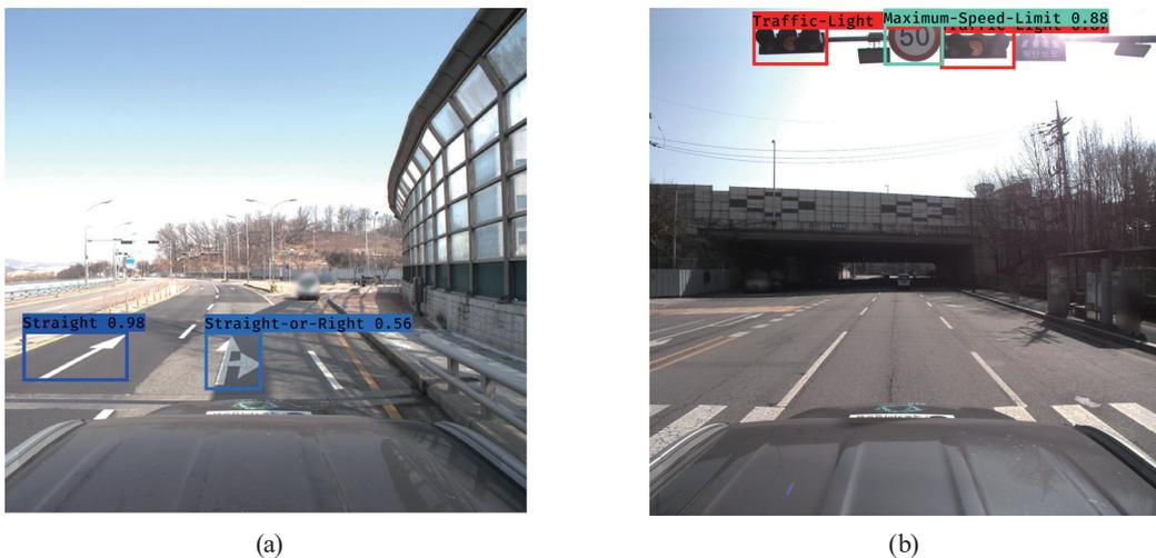
Fig. 5. (Color online) Road facilities detection: (a) straight and straight or right road marks and (b) traffic light and maximum speed limit sign.
