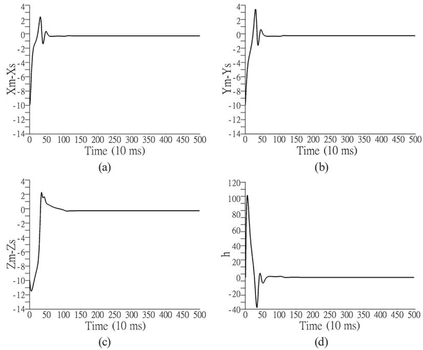
Fig. 1. Time series of (a)  $x_m - x_s$ , (b)  $y_m - y_s$ , (c)  $z_m - z_s$ , and (d)  $h$  of error dynamics of Lü chaotic systems with parameters  $x_m(0) = y_m(0) = z_m(0) = 0.1$ ,  $x_s(0) = y_s(0) = z_s(0) = 10$ ,  $h(0) = 0$ ,  $\alpha = 21$ , and coupling strength  $k = 440$  underlying the synchronization scheme with a dynamic controller.
