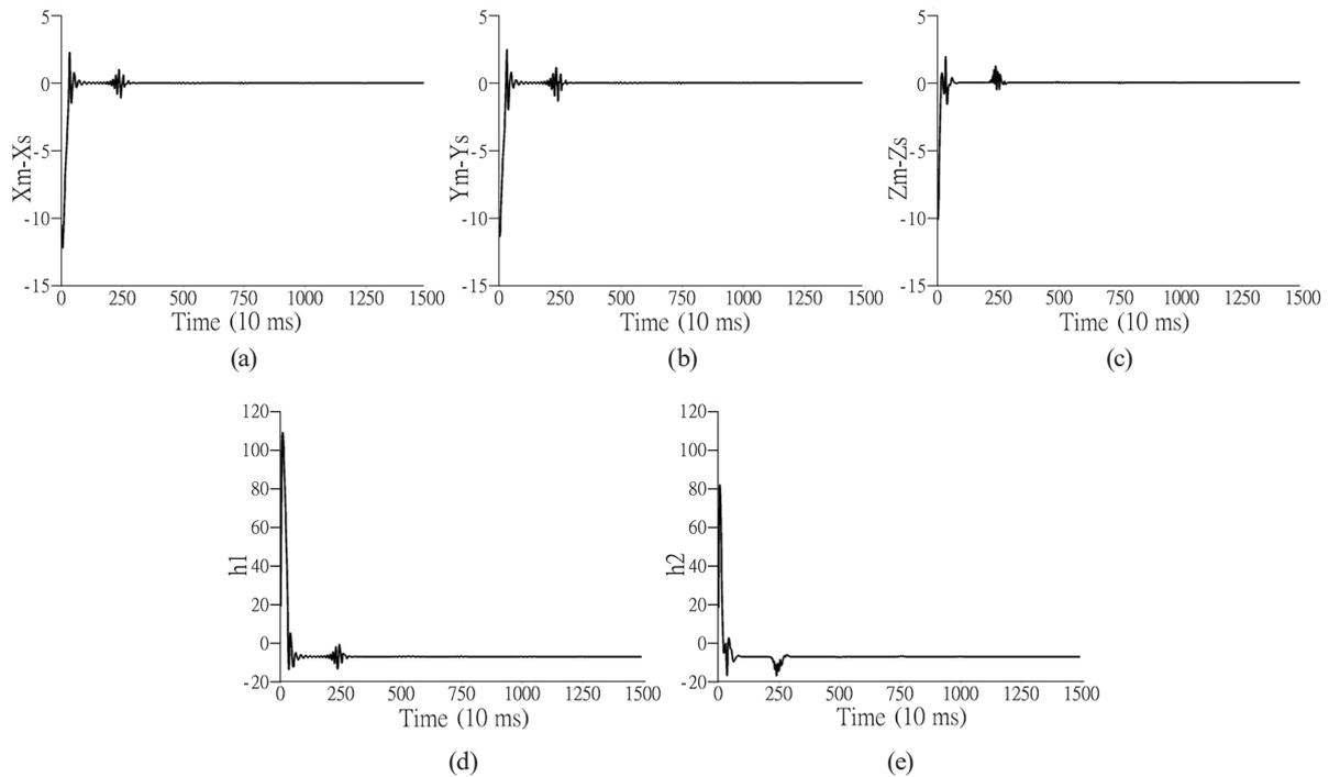
Fig. 2. Time series of (a)  $x_m - x_s$ , (b)  $y_m - y_s$ , (c)  $z_m - z_s$ , (d)  $h_1$ , and (e)  $h_2$ , of error dynamics of Lü-like chaotic systems with parameters  $x_m(0) = y_m(0) = z_m(0) = 0.1$ ,  $x_s(0) = y_s(0) = z_s(0) = 10$ ,  $h_1(0) = h_2(0) = 0$ ,  $\alpha = 21$ , and coupling strength  $k = 440$  underlying the proposed ameliorated synchronization scheme with dynamic controllers.
