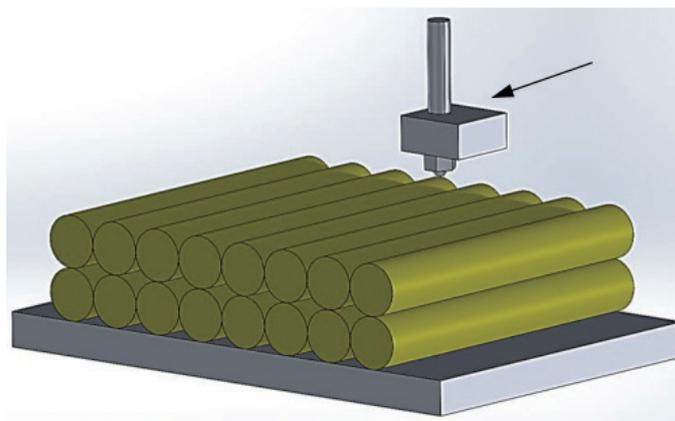
Fig. 1. (Color online) Schematic of the work theorem of FDM.
