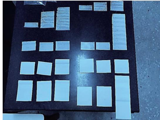
Fig. 7. (Color online) Nylon specimens 3D-printed at two different sizes (70 mm × 100 mm × x mm and 70 mm × 150 mm × x mm).
