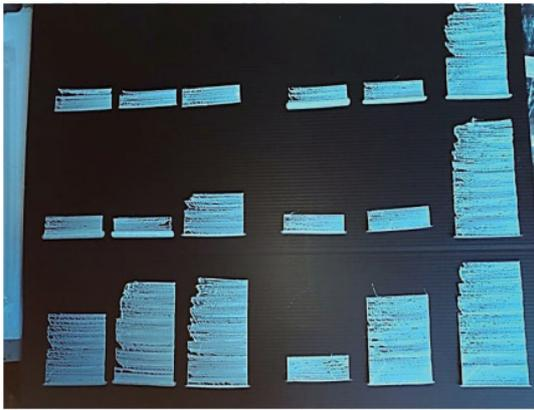
Fig. 6. (Color online) Nylon specimens 3D-printed at different speeds.
