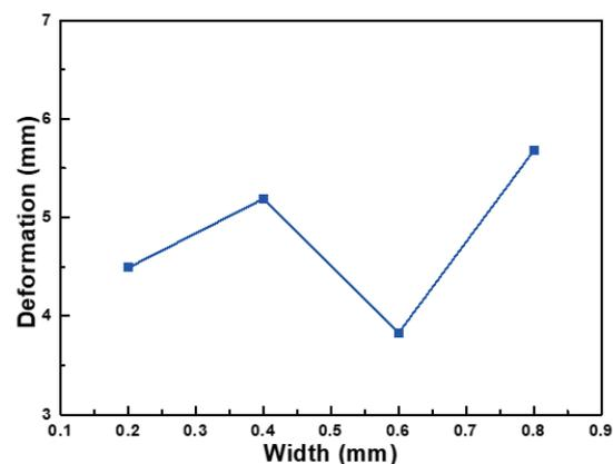
Fig. 5. (Color online) Variations in deformation value of printed nylon specimens with the size of  $70 \text{ mm} \times 150 \text{ mm} \times x \text{ mm}$  and with different  $x$  values.
