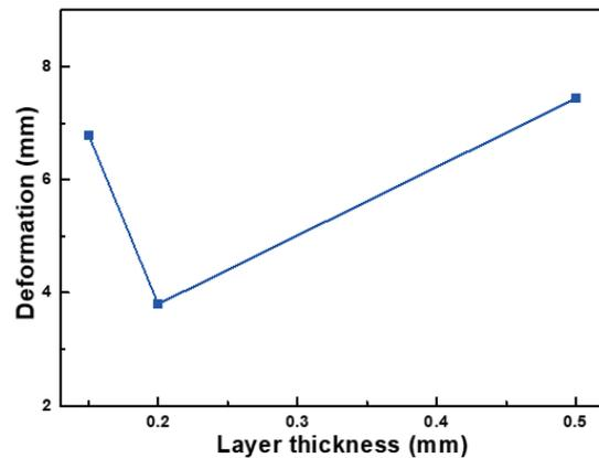
Fig. 3. (Color online) Variations in deformation value of nylon specimens printed with different layer thicknesses.
