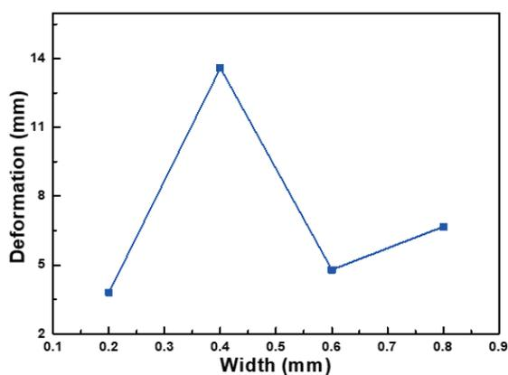
Fig. 4. (Color online) Variations in deformation value of printed nylon specimens with the size of  $70 \text{ mm} \times 100 \text{ mm} \times x \text{ mm}$  and with different  $x$  values.
