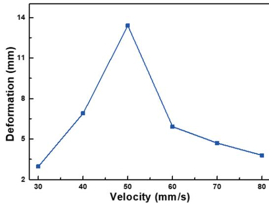
Fig. 2. (Color online) Variations in deformation value of nylon specimens printed at different printing speeds.
