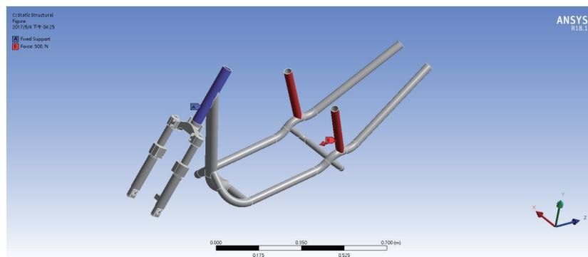
Fig. 13. (Color online) Boundary conditions of upper and lower bending moment stiffnesses.
