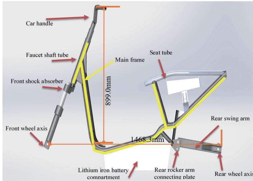
Fig. 1. (Color online) Structure of the 3D model for preliminary analysis.
