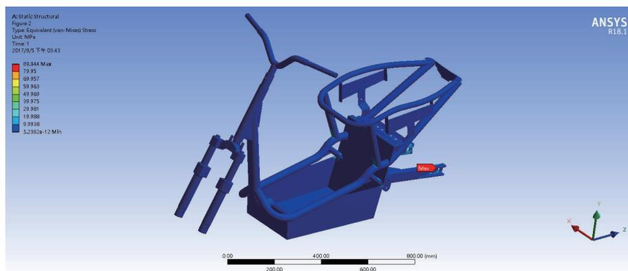
Fig. 5. (Color online) Reference point of the maximum stress position.
