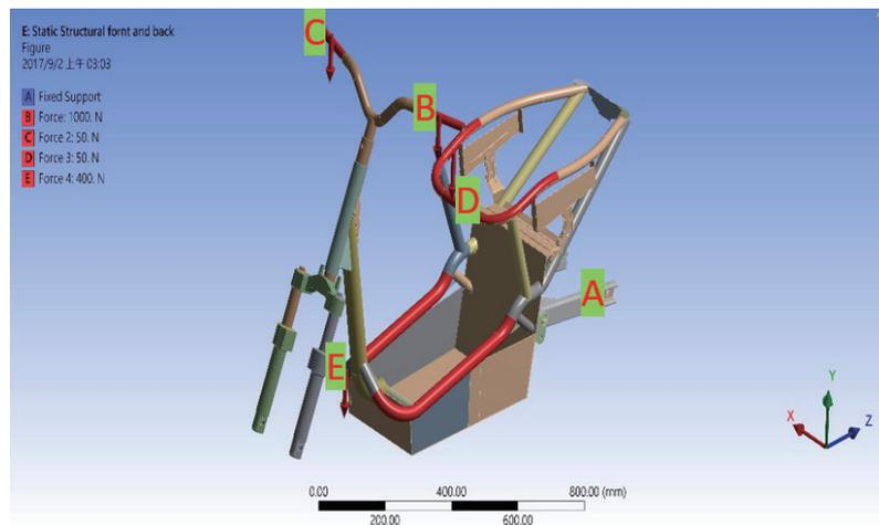
Fig. 9. (Color online) Boundary condition when rear wheel axle was constrained.
