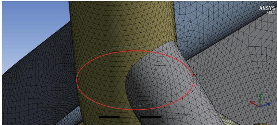
Fig. 3. (Color online) Densified area of mesh refinement at connection between head tube and main frame.
