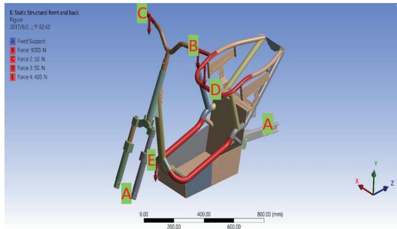
Fig. 11. (Color online) Boundary conditions when both front and rear wheel axle centers were constrained.
