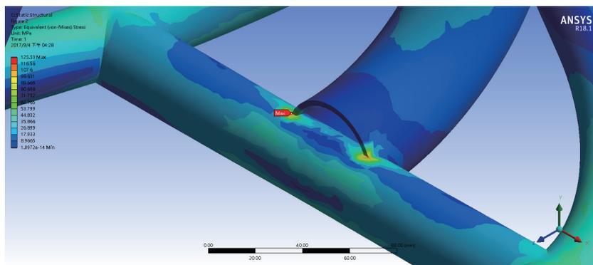
Fig. 16. (Color online) Positions of the maximum front and rear torque stresses.
