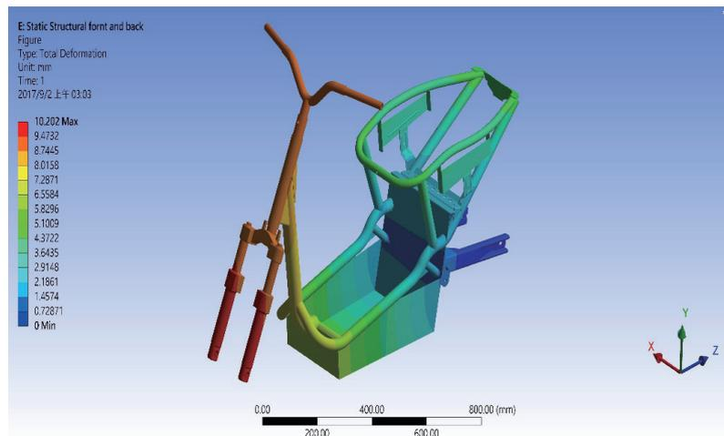
Fig. 10. (Color online) Axial force transmission path when rear wheel axle was constrained.
