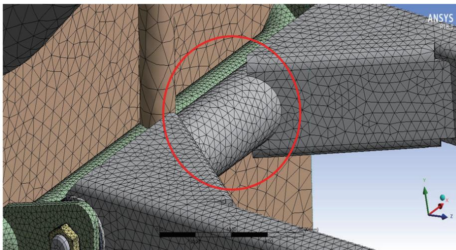
Fig. 4. (Color online) Densified area of mesh refinement at connection between main frame and seat tube.
