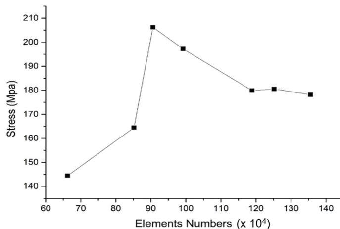
Fig. 6. Mesh convergence curve.
