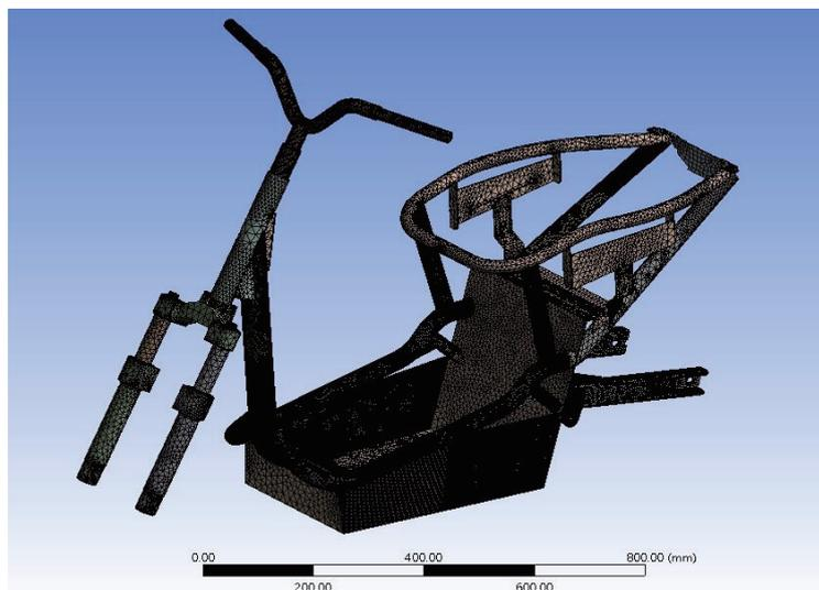
Fig. 2. (Color online) Grid of electric motorcycle frame.
