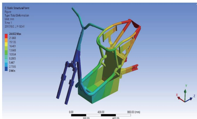
Fig. 8. (Color online) Force transmission path when the front wheel axle was constrained.
