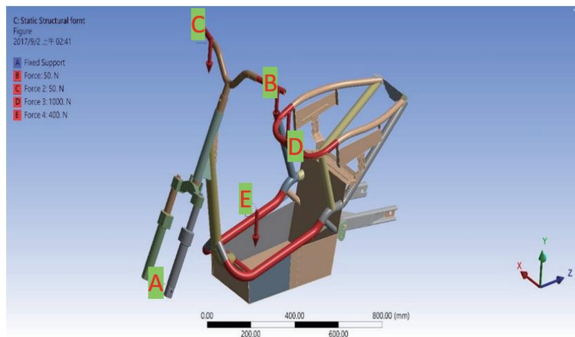
Fig. 7. (Color online) Boundary condition when front and rear wheel axles were constrained.
