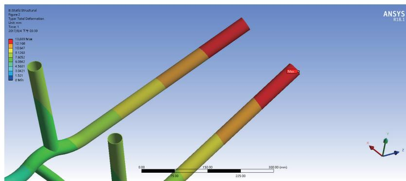
Fig. 15. (Color online) Positions of the maximum left and right bending moment deformations.
