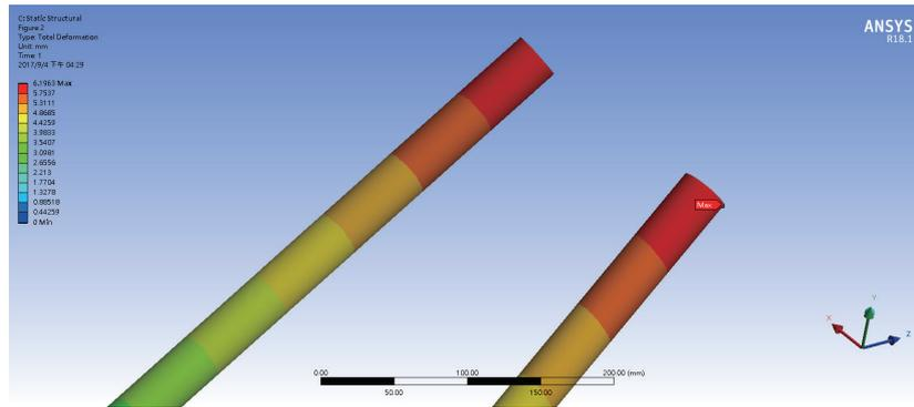
Fig. 14. (Color online) Positions of the maximum up and down bending moment deformations.
