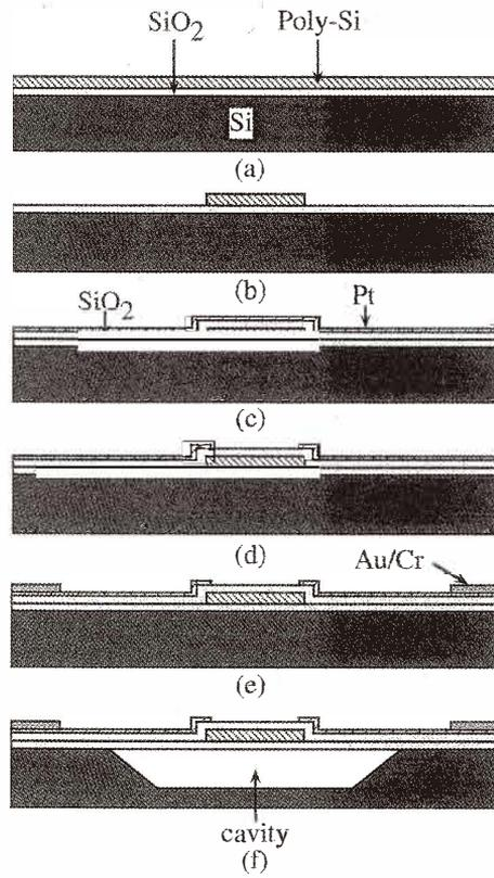
Fig. 1. Fabrication of the microheater.
