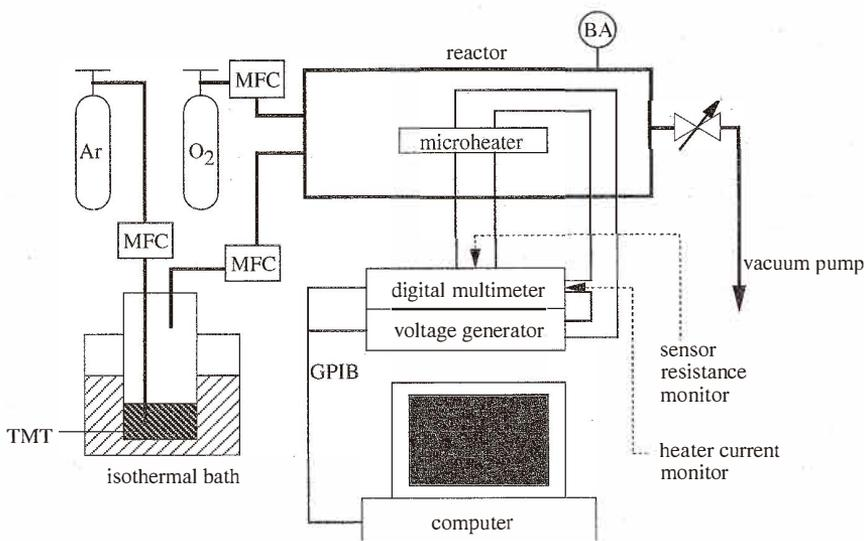
Fig. 3. A schematic diagram of the novel MOCVD system.
