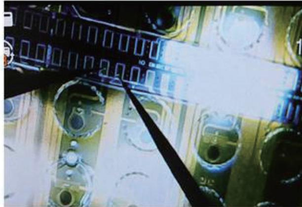
Fig. 3. (Color online) Probes come into contact with the input drive signal pads on the chip.
