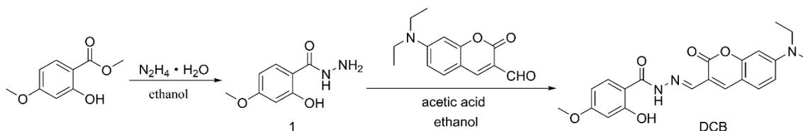
Fig. 1. Synthetic route to compound DCB.
