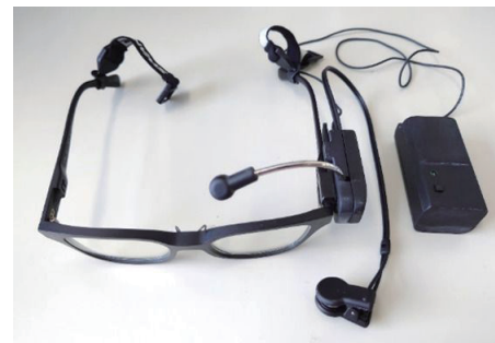
Fig. 6. (Color online) Spectacle-shaped EEG machine
