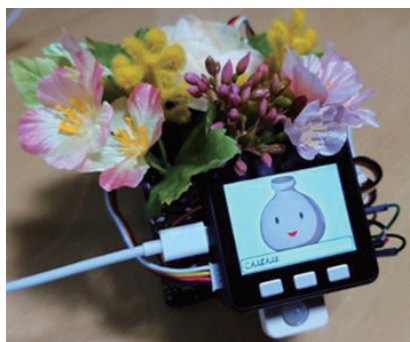
Fig. 4. (Color online) Picture of the developed flowerpot system.
