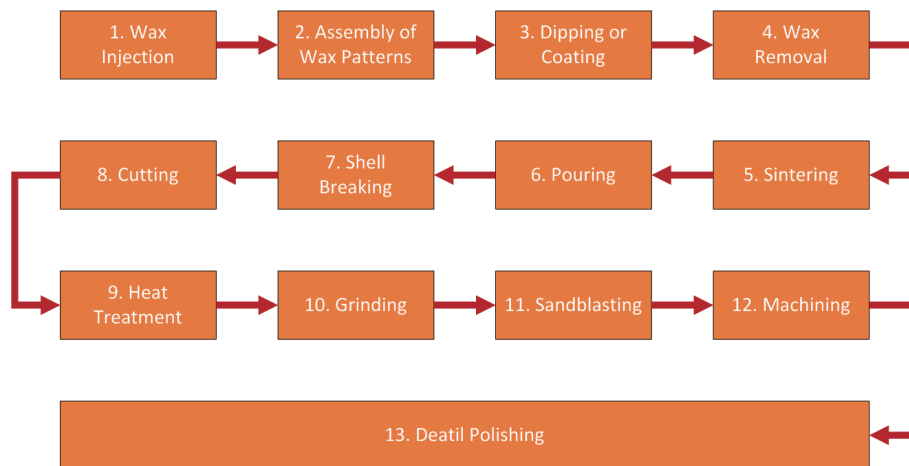
Fig. 1. (Color online) Flowchart of propeller precision casting.
