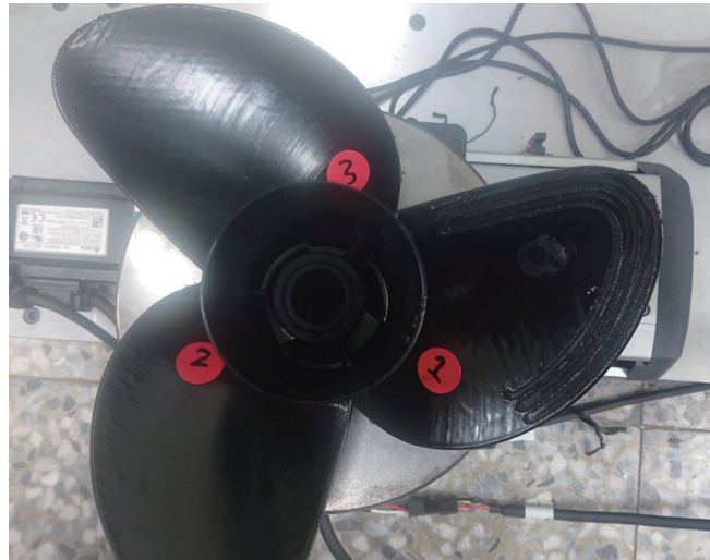
Fig. 15. (Color online) Additional coating applied to the workpiece.
