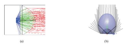
Fig. 2. (Color online) Lens design. (a) Plano-aspherical lens and (b) ray trace of freeform lens at cross section.
