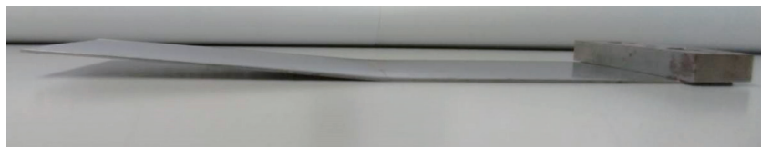
Fig. 4. (Color online) Deformation condition after direct energy deposition.
