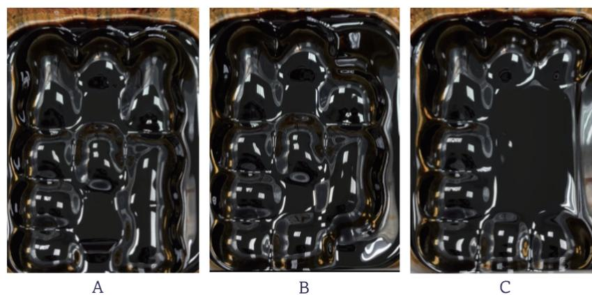
Fig. 10. (Color online) Display of letters “A”, “B” and “C” formed with tactile bulges.
