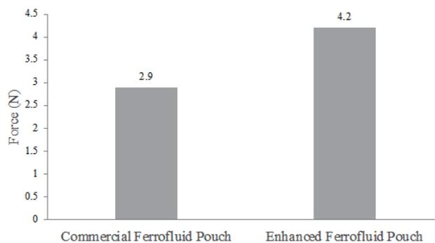
Fig. 4. Force feedback values of commercial and enhanced ferrofluid pouches.
