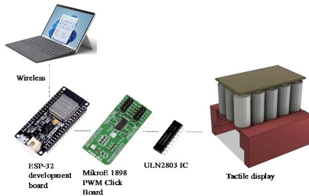
Fig. 3. (Color online) System architecture of wireless tactile display.
