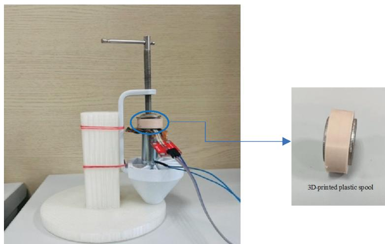
Fig. 1. (Color online) Experiment setup for measuring the force feedback.
