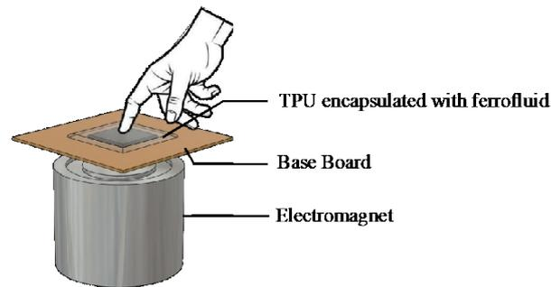
Fig. 2. (Color online) Schematic view of a single cell.
