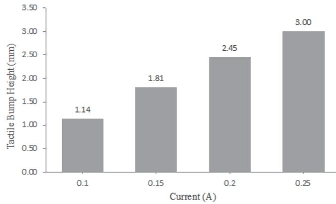
Fig. 6. Tactile bump height vs current.
