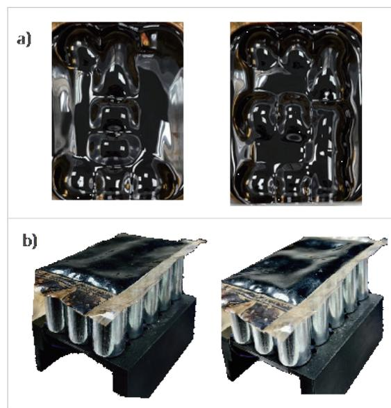
Fig. 9. (Color online) Display of numbers “1” and “3” formed with tactile bulges. (a) Without TPU pouch (top view). (b) With fluid-encapsulated TPU pouch (side view).
