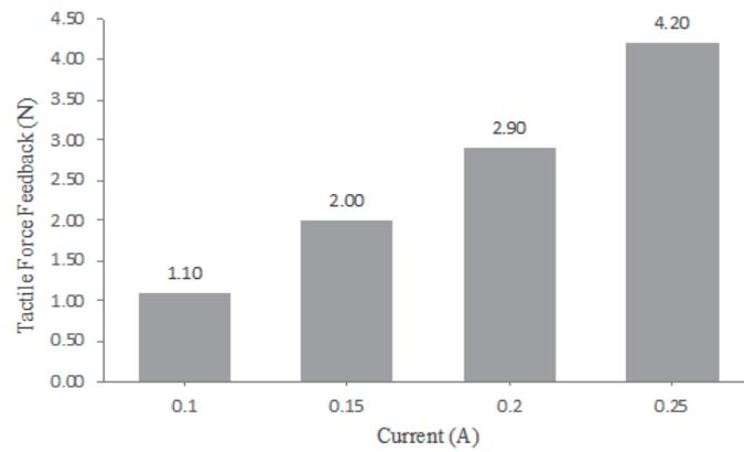
Fig. 7. Force feedback vs current.
