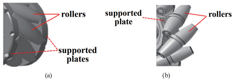
Fig. 9. (Color online) Placement types of rollers around wheel. (a) Two-ends-supported and (b) middle-supported types.
