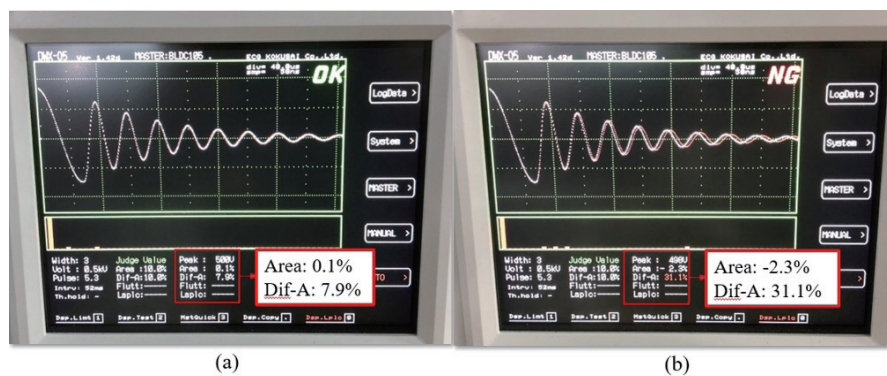
Fig. 8. (Color online) Photographs of layer short circuit measurement results of (a) normal and (b) abnormal stator coils.
