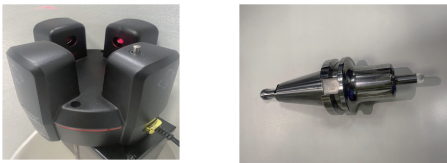
Fig. 1. (Color online) 3D sensing module and standard rod. (3)
