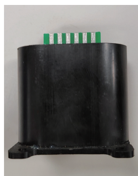
Fig. 7. (Color online) Fabricated gas detection module for carbon monoxide sensor based on composite electrochemical components.
