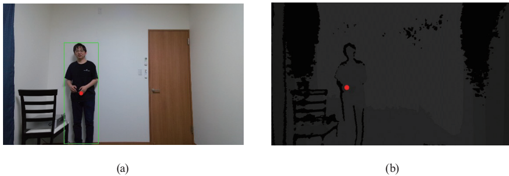
Fig. 7. (Color online) (a) Human detection result on RGB image. (b) Human detection result on aligned depth image.
