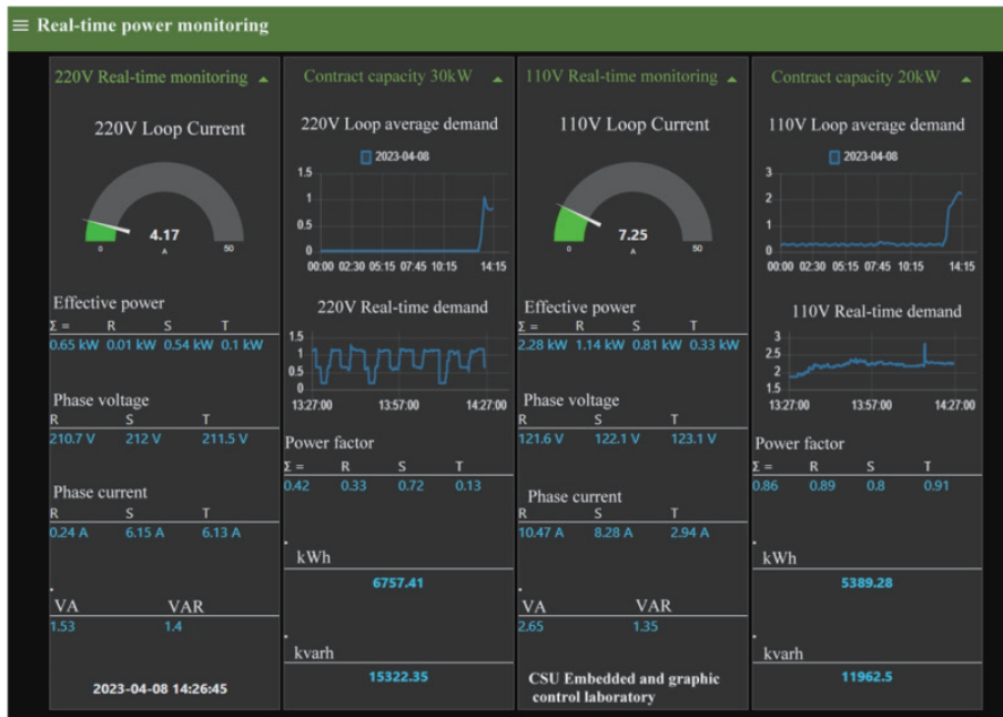
Fig. 17. (Color online) Real-time power monitoring screen for 220 and 110 V main circuit.
