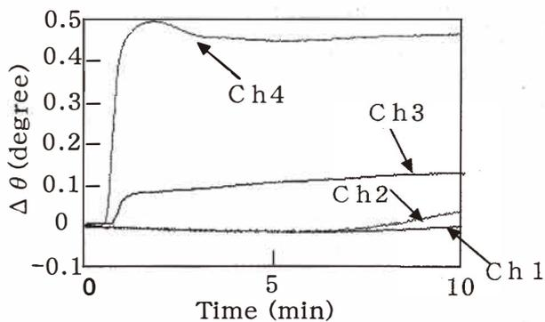
Fig. 9. Typical responses of each channel (Ch. 1–Ch. 4) of the SPR sensor to the *Gin-kouburi* sample, where distilled water was used as the reference liquid.
