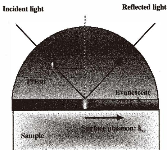
Fig. 1. Kretschmann-type SPR configuration.
