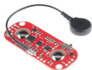
Fig. 3. (Color online) MyoWare Muscle Sensor module.
