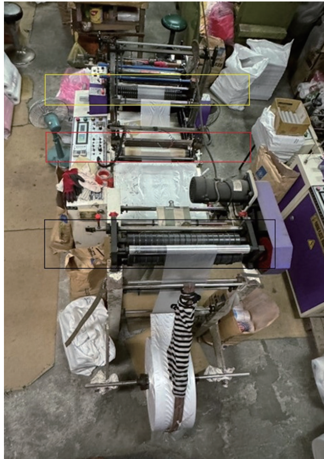
Fig. 4. (Color online) Aerial view of a roll-to-roll plastic bag processing machine.
