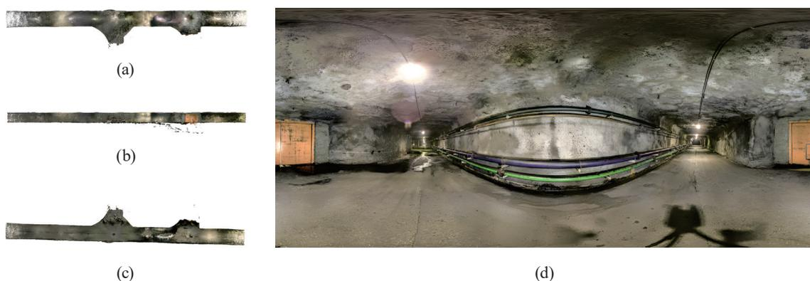
Fig. 4. (Color online) Effect of each viewpoint of the underground tunnel data. (a) Top, (b) side, and (c) elevation views of the point cloud. (d) Internal.
