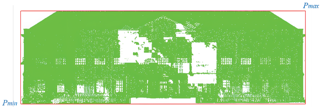
Fig. 5. (Color online) Minimum external bounding box of original point cloud.
