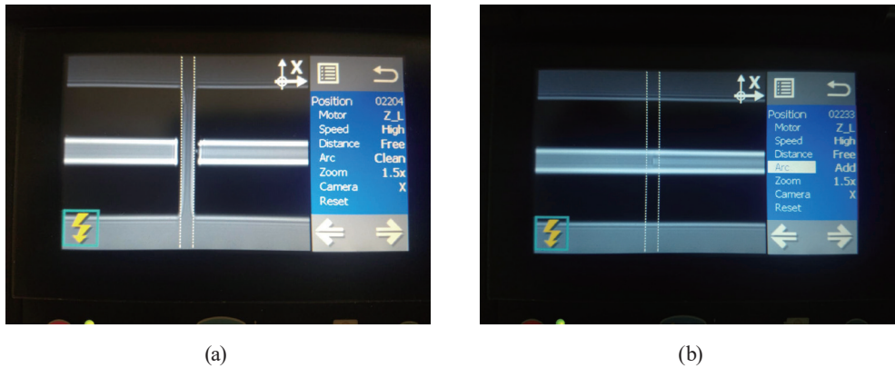
Fig. 2. (Color online) (a) CL fiber (left-hand side) and SMF (right-hand side) before splicing, and (b) CL fiber and SM28 after splicing.
