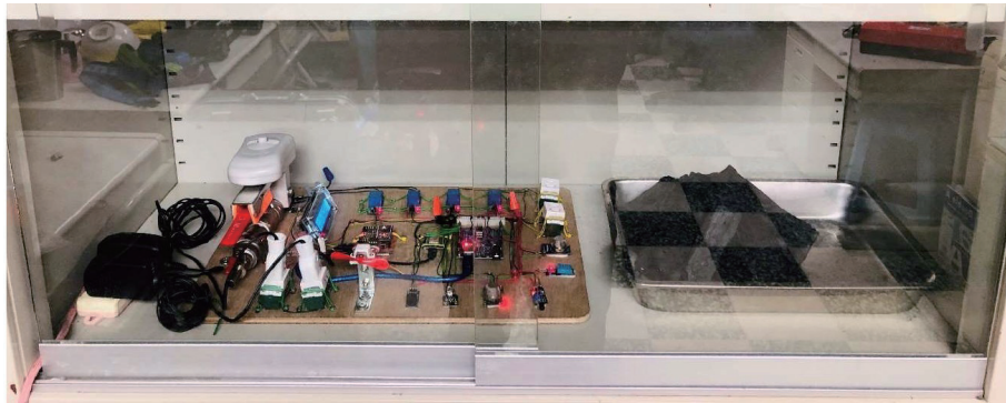
Fig. 3. (Color online) Enclosed space for simulating CO detection.
