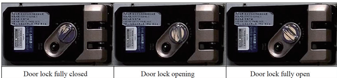
Fig. 10. (Color online) System activating electronic door lock opening function.
