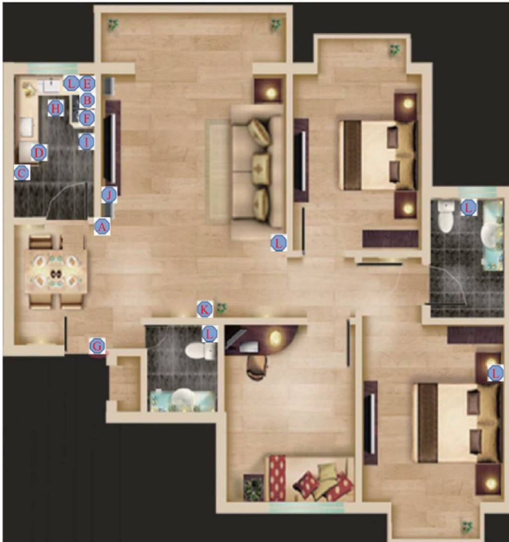
Fig. 21. (Color online) Recommended installation locations for elderly smart home safety devices diagram.
