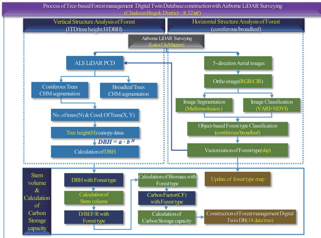
Fig. 11. (Color online) Process of tree-based forest management digital twin database construction with airborne LiDAR surveying data (Chiaksan Bugok District: 8.32 km<sup>2</sup>).
