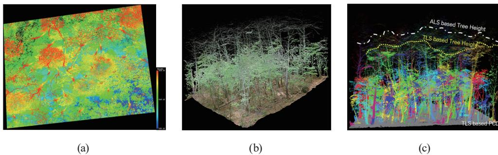
Fig. 6. (Color online) TLS-based point cloud data of Plot 2: (a) TLS-based 2D point cloud data (Plot 2: BLK2GO), (b) TLS-based 3D point cloud data (Plot 2: BLK2GO), and (c) difference in tree height (ALS VS TLS).
