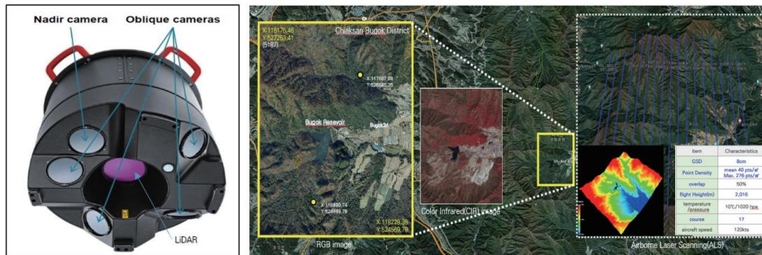
Fig. 4. (Color online) Data acquisition with airborne LiDAR photogrammetry.
