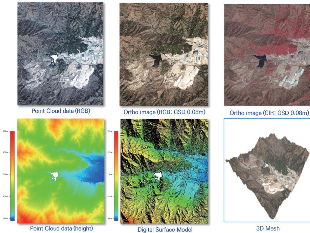
Fig. 5. (Color online) Outputs with CV analysis of five-direction aerial images.
