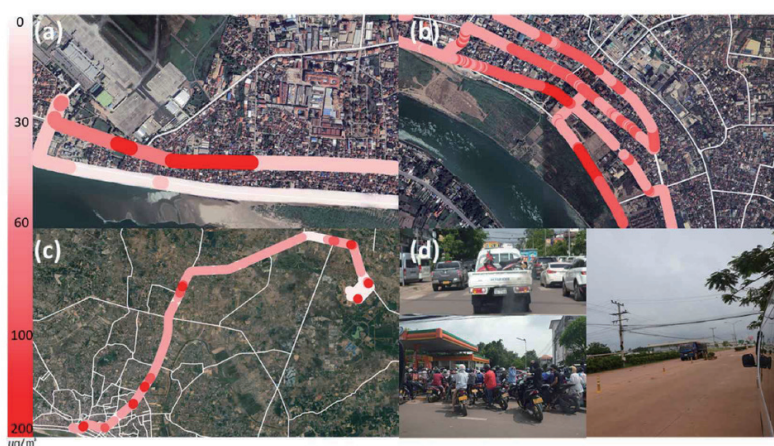
Fig. 2. (Color online) Sniffer4D 2D maps in the road around (a) Wattay International Airport, (b) the city, (c) VITA industrial areas, and (d) local on-site emissions during measurements.
