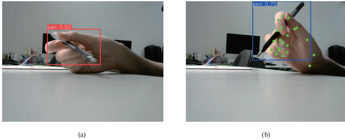
Fig. 11. (Color online) Detection results with and without hand skeleton points.
