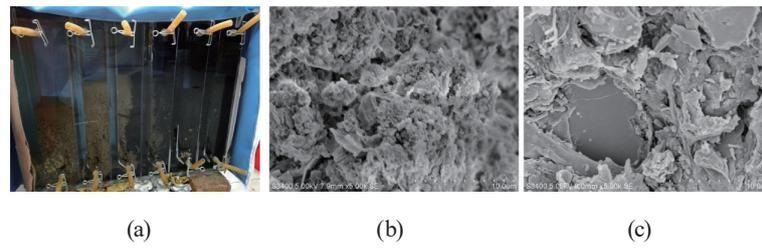
Fig. 3. (Color online) SEM images of sludges in initial period (24 d): (a) in ABR, (b) brown-yellow sludge, and (c) black sludge.
