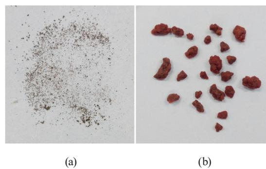
Fig. 5. (Color online) Comparison of sludge colors observed (a) before (0 d) and (b) after treatment for 150 d.
