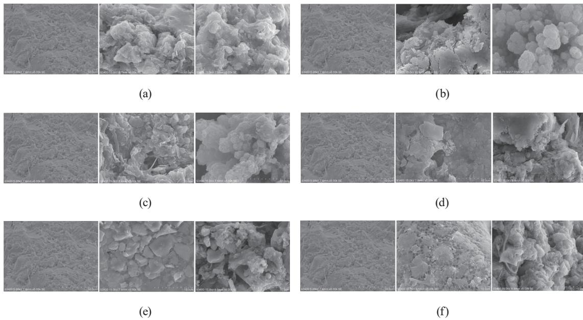
Fig. 4. SEM images of anaerobic activated sludge in compartments on (left) 0th, (middle) 68th, and (right) 150th days. Compartments (a) 1, (b) 2, (c) 3, (d) 4, (e) 5, and (f) 6.
