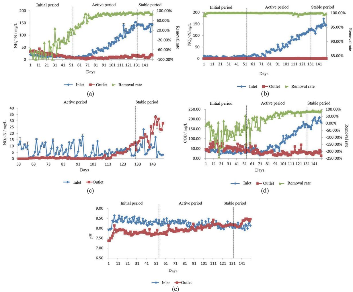
Fig. 2. (Color online) Concentrations and removal rates of (a)  $\text{NH}_4^+\text{-N}$ , (b)  $\text{NO}_2^-\text{-N}$ , (c)  $\text{NO}_3^-\text{-N}$ , (d) COD, and (e) pH in each period of experiment.
