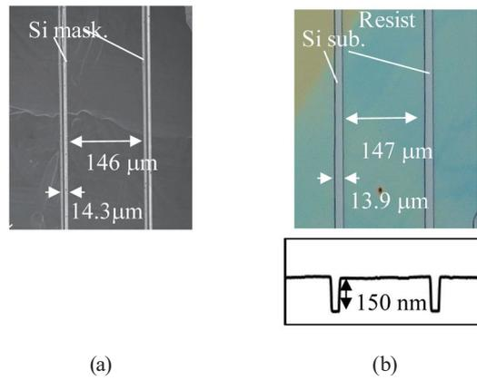
Fig. 5. (Color online) (a) SEM image of fabricated micrometer-sized stencil mask. (b) Optical microscopy image of resist pattern after exposure and development and cross-sectional profile.
