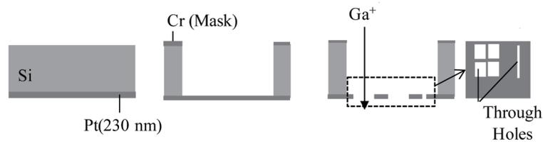
Fig. 4. (Color online) Fabrication of stencil masks with a Pt film structure.
