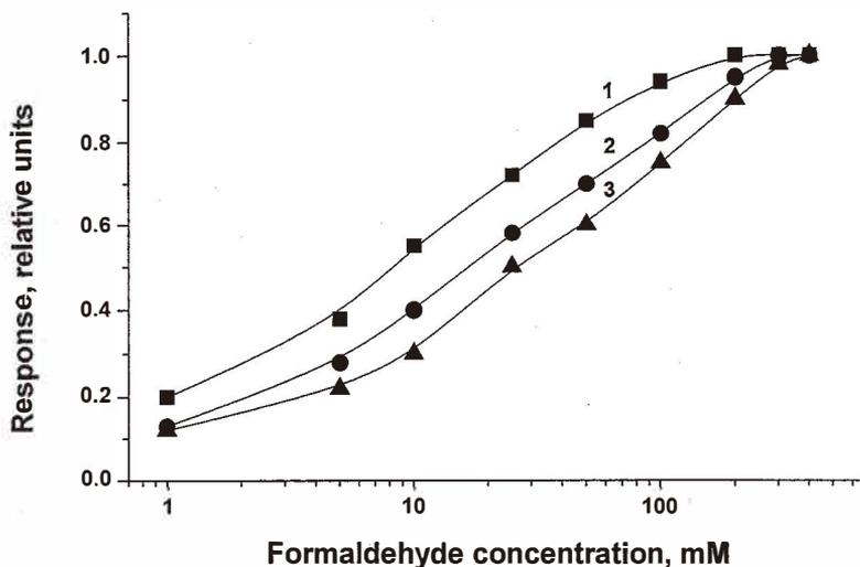
Fig. 2. Calibration curves (in semilogarithmic scale) for formaldehyde specific amperometric (1), conductometric (2) and potentiometric (3) biosensors as measured in a 10 mM phosphate buffer, pH 7.7.
