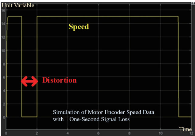
Fig. 8. (Color online) MATLAB simulation of motor encoder speed data with one-second signal loss.
