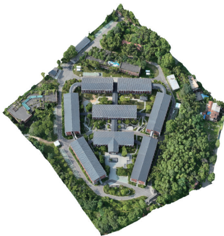
Fig. 14. (Color online) Trimmed tilted mesh model.
