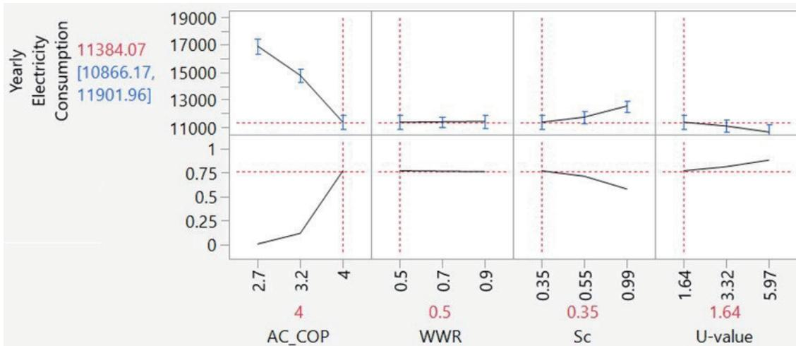
Fig. 12. (Color online) DSD model optimization using profiler tool in JMP software.
