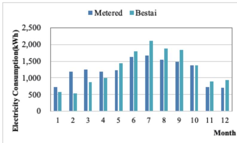
Fig. 8. (Color online) Comparison of monthly electricity consumption with metered and simulated tools.
