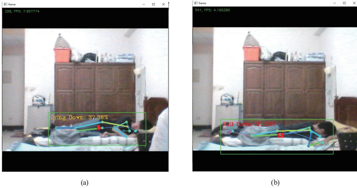
Fig. 10. (Color online) (a) Experimental result where AI identifies image as "Lying Down," displaying orange warning and showing accuracy. (b) Experimental result where AI identifies image as "Fall Down," displaying red warning and showing accuracy.
