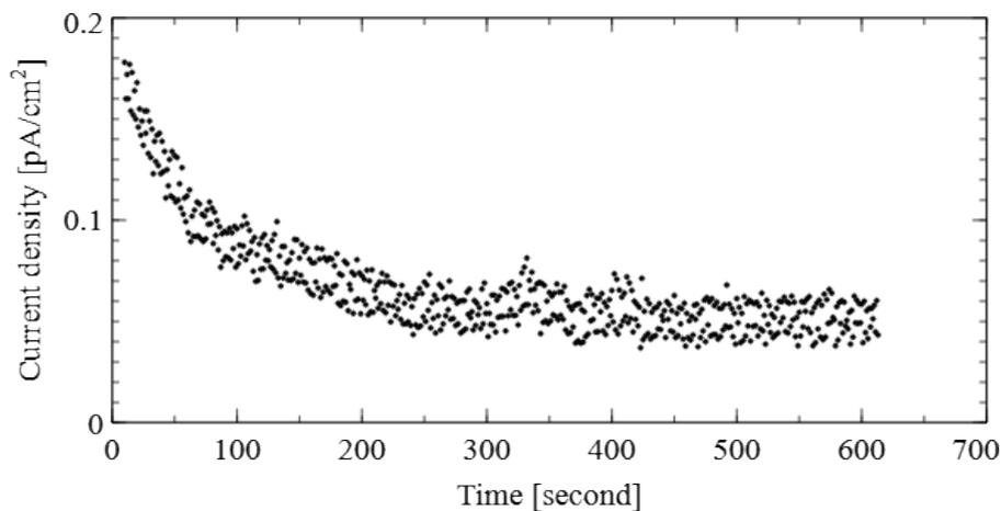
Fig. 3.  $J$ – $t$  characteristics during discharge at  $0$  V.
