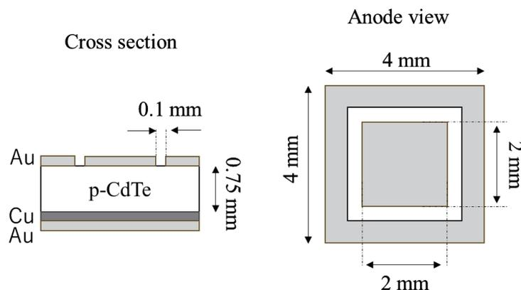
Fig. 1. Structure of fabricated Cu–CdTe detectors.
