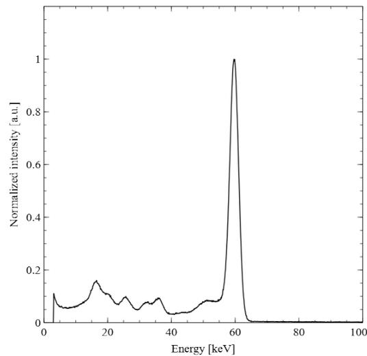
Fig. 7. Measurement result of  $\gamma$ -ray spectrum of  $^{241}\text{Am}$  using aged Cu–CdTe detector biased at  $-900\text{ V}$ .
