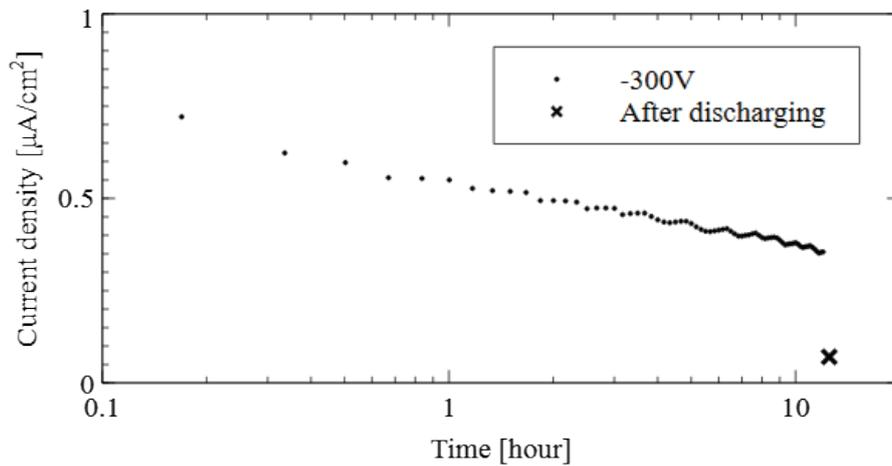
Fig. 2.  $J$ – $t$  characteristics of Cu–CdTe detector during electrical aging at  $-300$  V.
