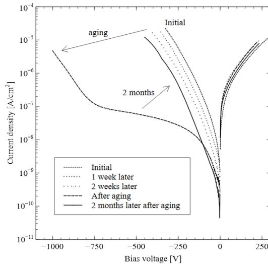
Fig. 6.  $J$ - $V$  characteristics of another Cu-CdTe detector before and after aging.
