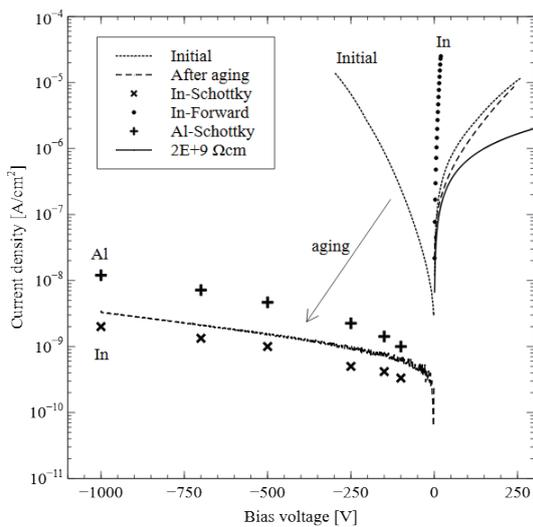
Fig. 4.  $J$ - $V$  characteristics of Cu-CdTe detector before and after electrical aging.
