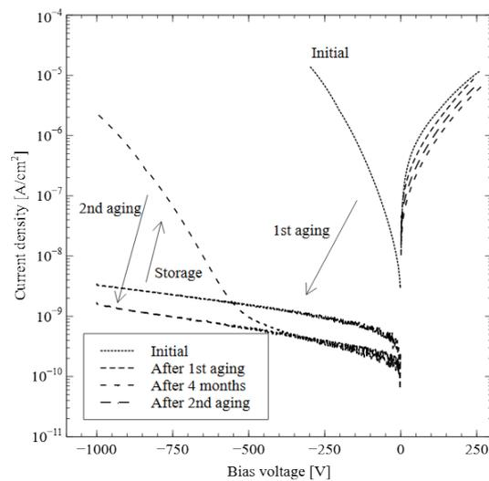
Fig. 5.  $J$ - $V$  characteristics of Cu-CdTe detector after four months of storage and after second aging.
