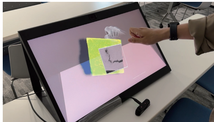
Fig. 13. (Color online) Experimental conditions: the observer moves and rotates 3D objects and boundaries with hand movements. By changing the position of the observed cross section, the complex structure of the casting cavity can be understood spatially.
