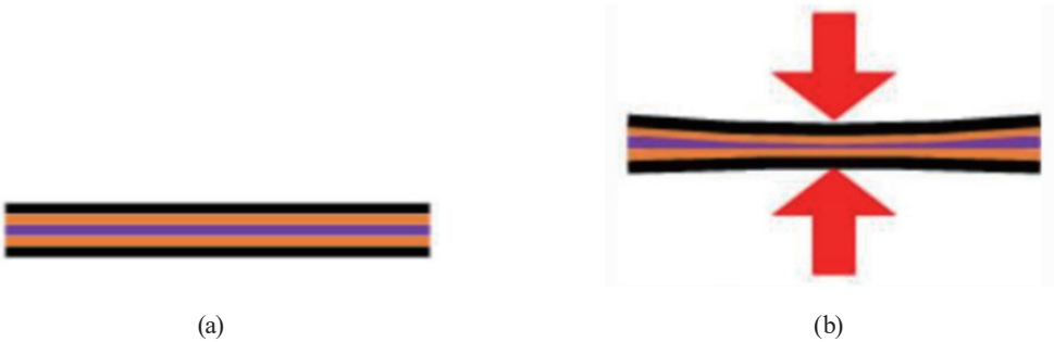
Fig. 5. (Color online) Operation of pressure sensor based on piezoresistive effect. (a) Internal structure of sensor (the orange line represents the circuitry and the purple line represents the piezoresistive material). (b) Pressure decreases the resistance of the piezoresistor.
