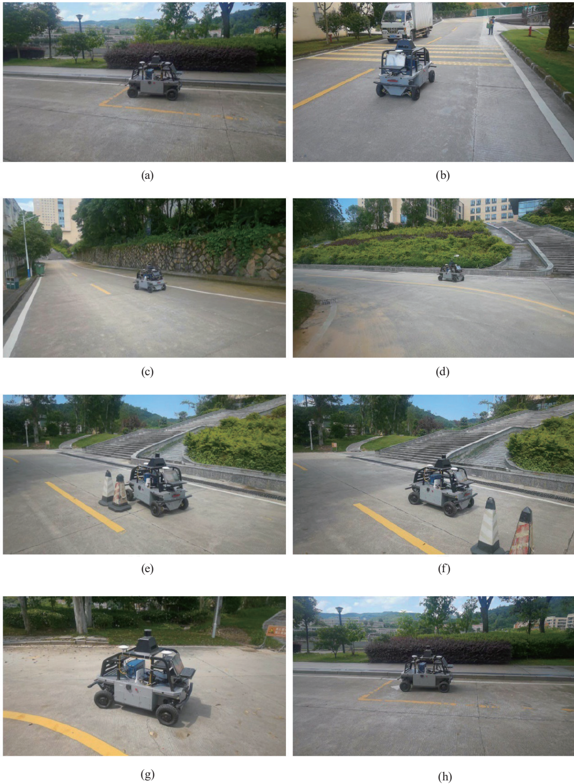
Fig. 18. (Color online) Test of real-vehicle cruise driving: (a) getting started, (b) straight-line deceleration, (c) straight-line acceleration, (d) turning left, (e) obstacle avoidance, (f) returning, (g) turning left, and (h) stopping.
