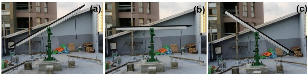
Fig. 7. (Color online) Automatic tracking and rotating mechanism: (a) mechanism tilt angle of  $26^\circ$ , (b) mechanism tilt angle of  $0^\circ$ , and (c) mechanism tilt angle of  $-26^\circ$ .
