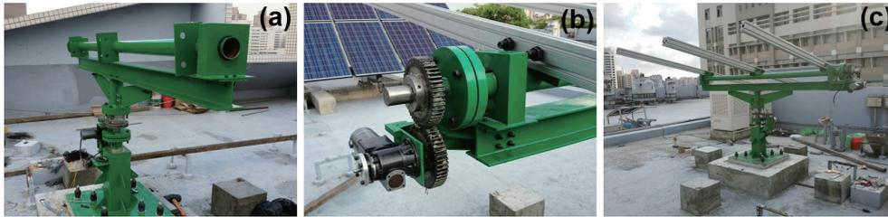
Fig. 5. (Color online) (a) Assembly of rotation structure, (b) assembly of drive mechanism, and (c) completed assembly of tracking system mechanism.
