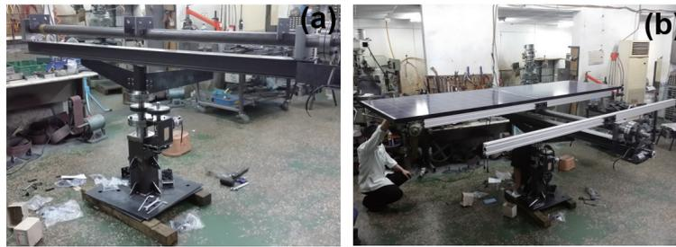
Fig. 4. (Color online) Pre-assemblies of (a) elevation rotation mechanism and (b) solar panel truss.
