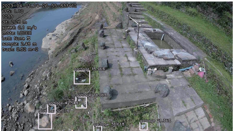
Fig. 21. (Color online) Qixian Bridge-Keelung River real-time garbage identification results_3.
