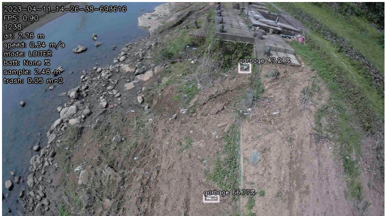
Fig. 20. (Color online) Qixian Bridge-Keelung River real-time garbage identification results_2.
