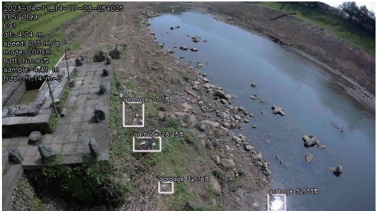
Fig. 19. (Color online) Qixian Bridge-Keelung River real-time garbage identification results_1.
