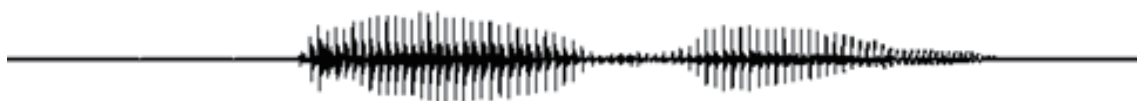
Fig. 4. Sample recorded waveform of the specific Mandarin phrase “导航”, which means “to navigate” in English, uttered by each speaker for speaker recognition (clean speech).
