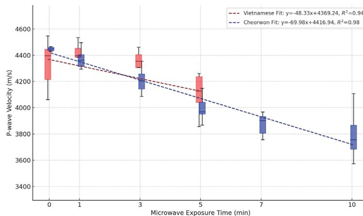
Fig. 3. (Color online) P-wave velocity variations with microwave exposure time for Cheorwon and Vietnamese basalt specimens.
