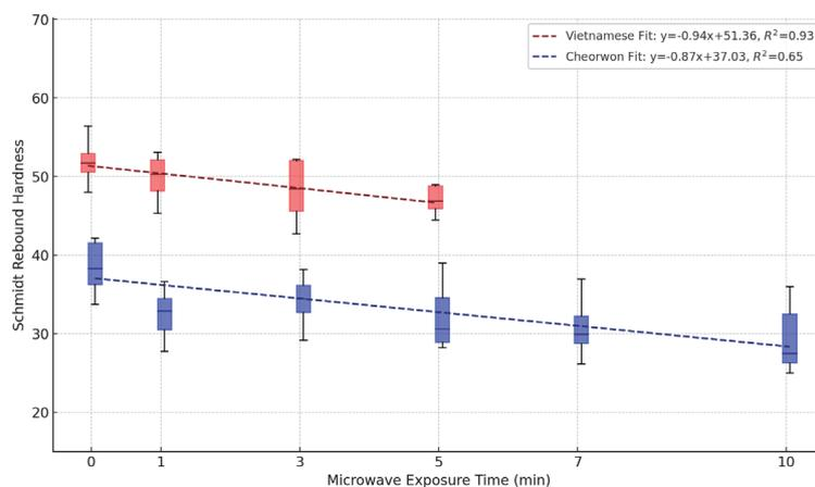
Fig. 4. (Color online) Schmidt rebound hardness variations with microwave exposure time for Cheorwon and Vietnamese basalt specimens.
