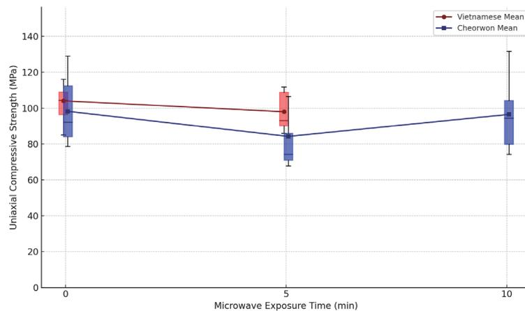
Fig. 6. (Color online) UCS variations with microwave exposure time for Cheorwon and Vietnamese basalt specimens.
