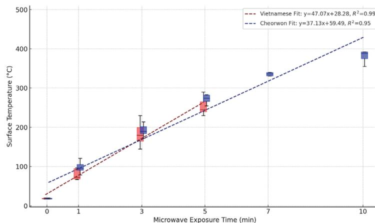
Fig. 2. (Color online) Surface temperature rise as a function of microwave exposure time for Cheorwon and Vietnamese basalts.
