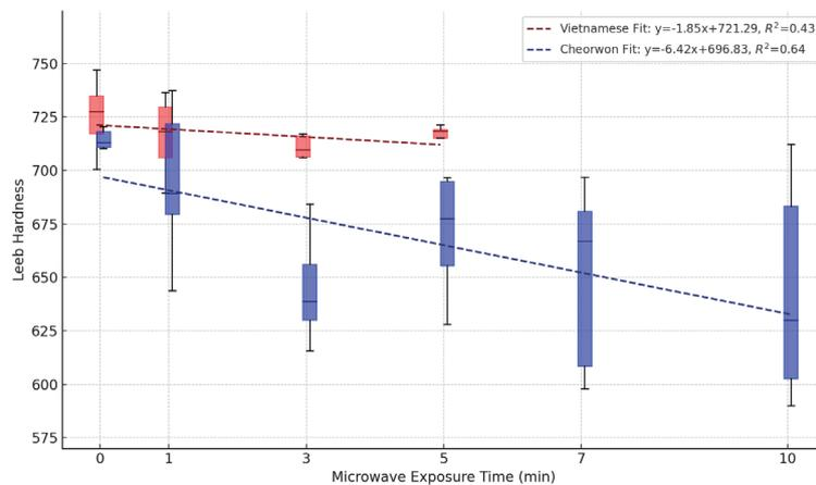
Fig. 5. (Color online) Leeb hardness variations with microwave exposure time for Cheorwon and Vietnamese basalt specimens.
