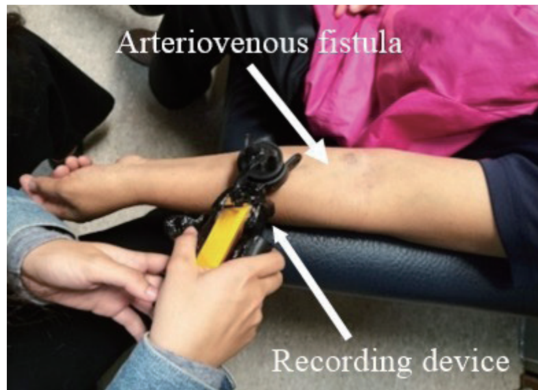
Fig. 2. (Color online) Operational process of the developed recording device.
